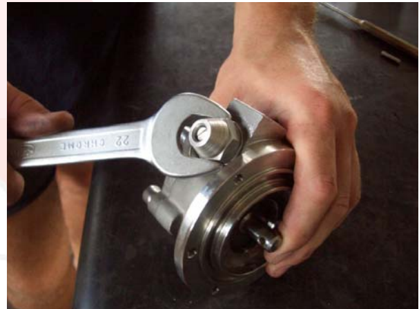
13) Remove hex nut from pump casing and pull out by-pass components.
