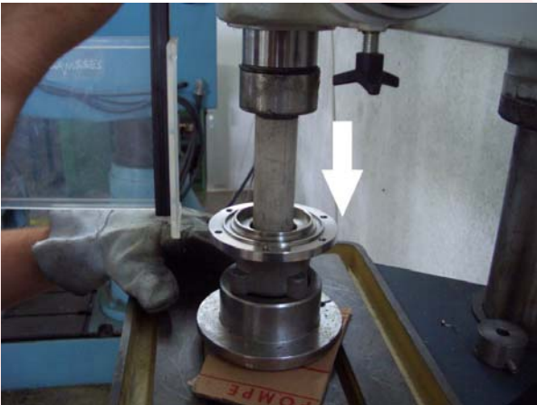
12) Disassembling cartridge make attention to not loose the small pins inside the hole's shaft.
