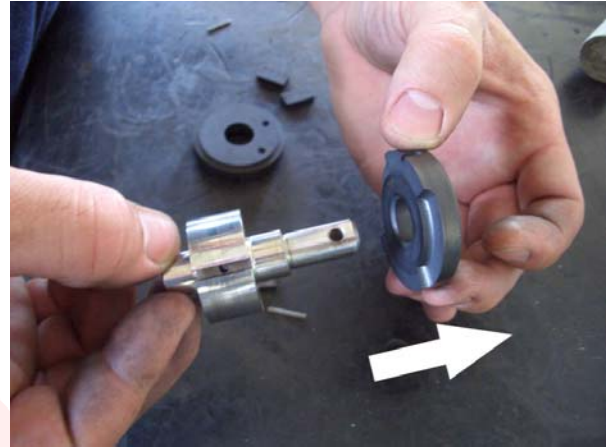
13) Remove hex nut from pump casing and pull out by-pass components.
