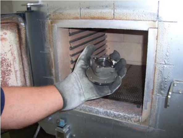
11) Then you can easily pull out the cartridge from the pump casing.
