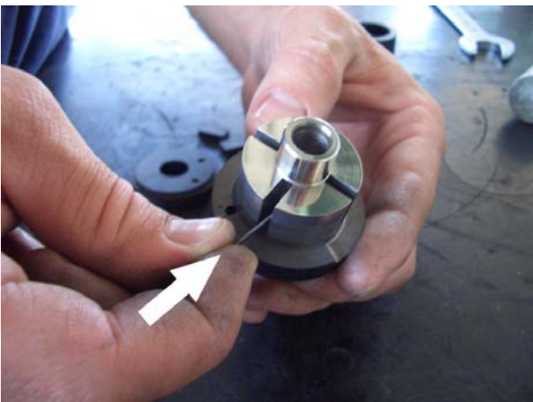
12) Disassembling cartridge make attention to not loose the small pins inside the hole's shaft.
